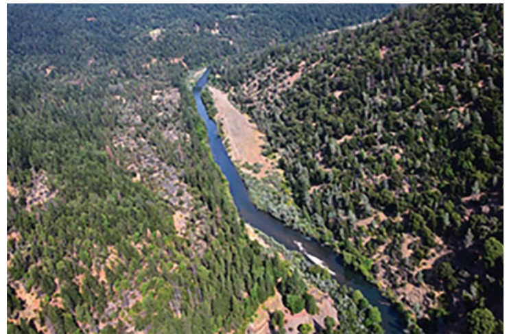
Figure 2. Looking downstream at the top-end of Dutch Creek project site in 2016. The strip of land terraced above the river on the right side of the photo largely contains non-native grasses and rarely connects to the river. The area was lowered so that it reconnects to the river at much lower flows to provide critical salmon habitat.
